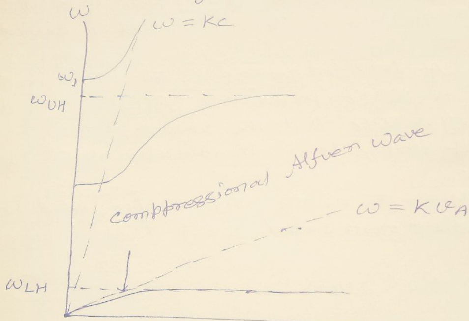
Dispersion for a wave propagating perpendicular to the magnetic field in a magnetized plasma.
